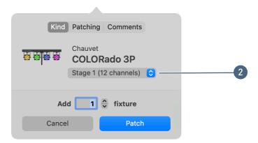
2 If the fixture has different operation modes (or "personalities"), select a mode from the menu below the fixture name. Be sure to select the same mode as on the fixture, or Lightkey will not be able to control the fixture! If no menu is shown then the fixture has no modes.
