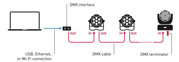
Each daisy chain of fixtures forms a **DMX universe** which operates up to 512 channels. For many installations a single universes is sufficient, but Lightkey can control up to eight full universes or 4096 channels.
