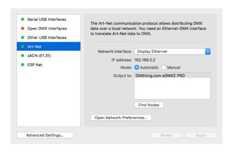
In most cases Lightkey can find connected Art-Net nodes automatically. If Lightkey can't find the node it often helps to connect it directly to your computer using an Ethernet cable in order to rule out network problems.
